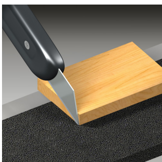
Figure 3: To accommodate setting blocks, notch out tape
